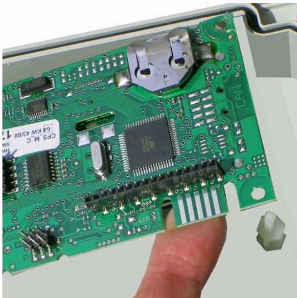
Lift the circuit board from the clasps
